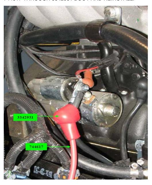
REMOVE OLD CABLE FROM ISOLATOR AND RED BOOT. REPLACE WITH NEW 744617. ROUTE CABLE THROUGH RED BOOT AND MOUNT TO INSOLATOR DISTRIBUTION POINT (3400071)
